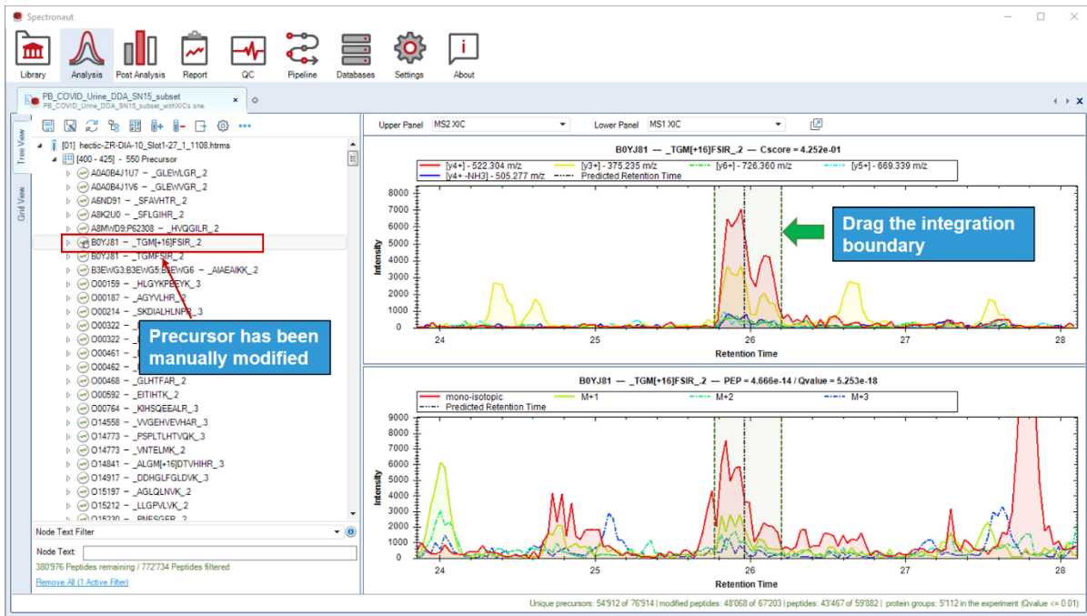
Figure 25. Reviewing Spectronaut peak picking. Integration boundaries can be modified by dragging them. The precursor will be marked as manually modified.
