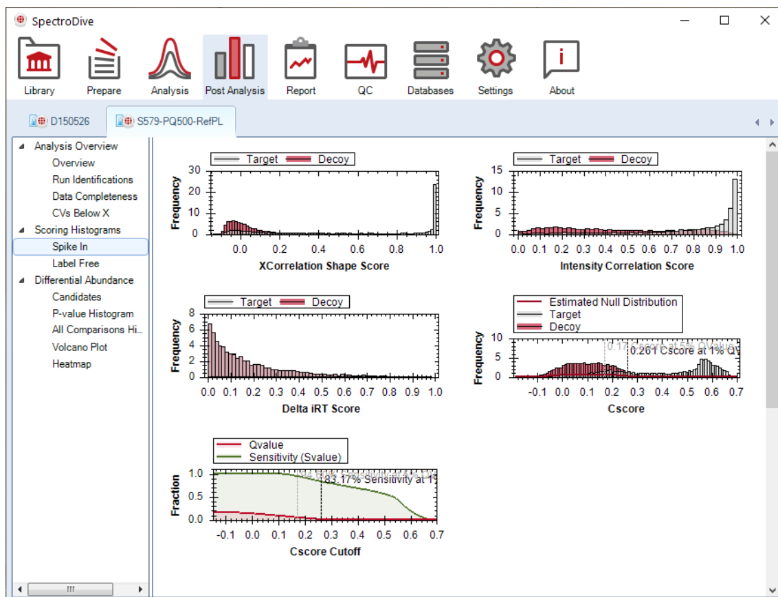
Figure 28. Post Analysis Perspective. Several summaries, tables and plots are available as you navigate through the nodes in the tree. On the figure a view of the scoring histograms for the spike-in peptides is displayed.
